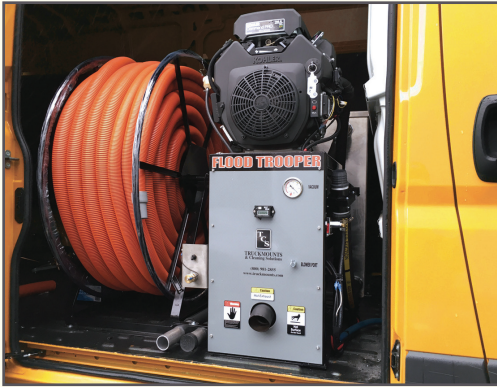
Dual Wand Upgrade Kohler 26.5 EFI - 4L DSL Blower
